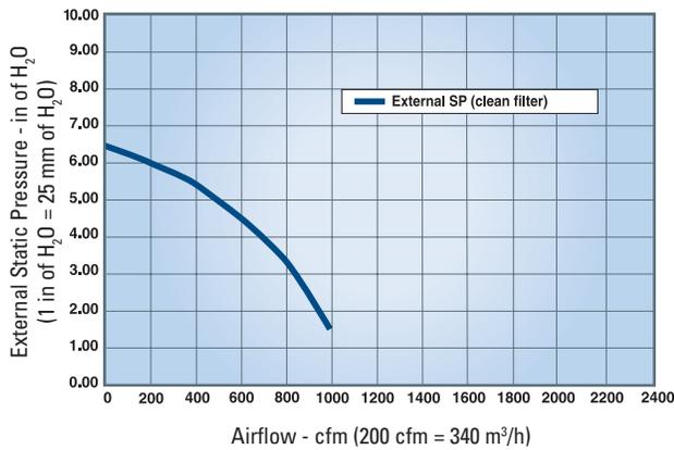
**DFO 1-1** 1.1kW 50Hz with 6" (152.4 mm) inlet duct (clean filter)
