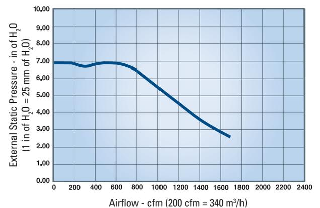
**DFO 3-3** 5HP 60Hz with 9" (228.6 mm) inlet duct (clean filters)
