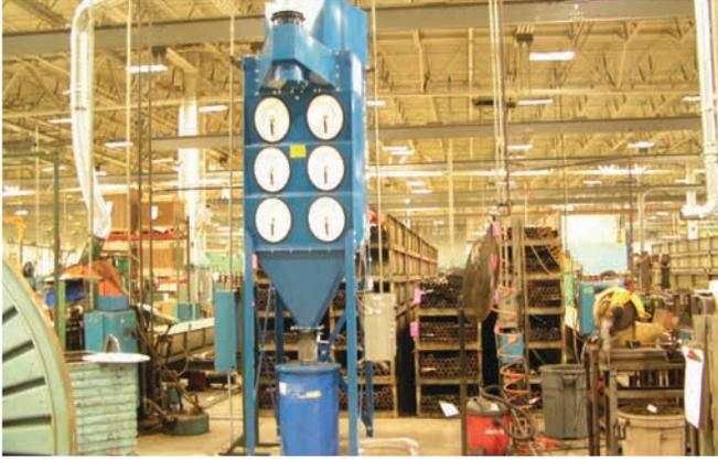
**DFO 3-6 on Sawing of High Pressure Hydraulic Hose**
