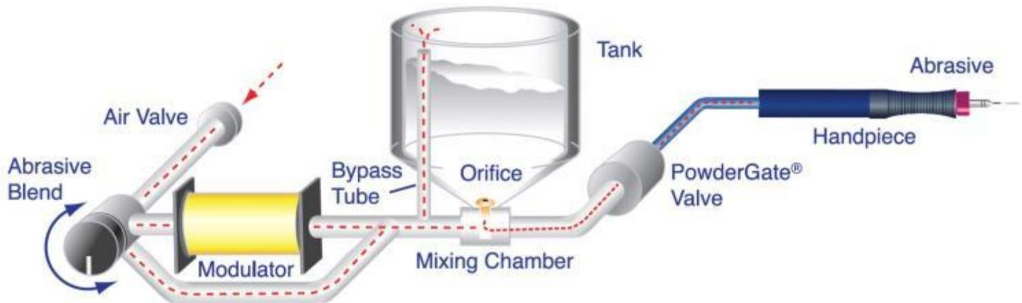
Step on the footswitch and the modulator opens and closes 50 or 60 times per second (depending on local power supplied at 50Hz or 60Hz), producing pulses in the air stream. The rapid change in air pressure fluidizes the abrasive above the orifice. The powder is then drawn through the orifice into the mixing chamber where it enters the air stream and exits the AccuFlo® through the PowderGate® valve traveling out to the nozzle.
