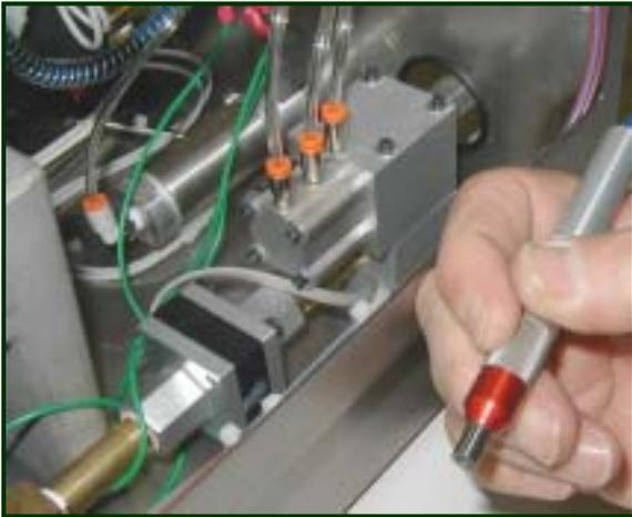
An exclusive feature of the DirectFlo and PowerFlo, Comco's PowderGate controls the abrasive flow internally, rather than relying on pinching a section of hose.
