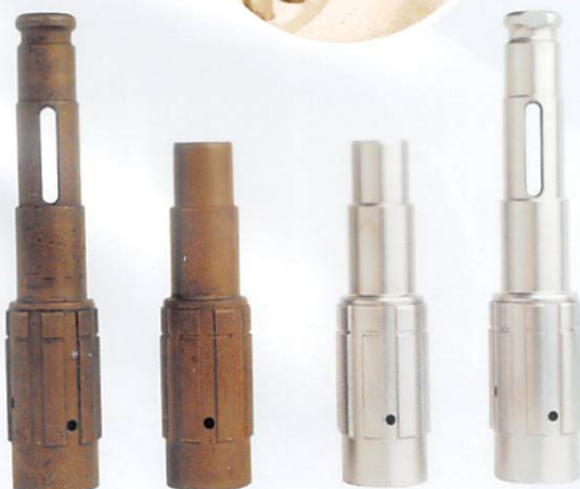
Before and after samples of the surface finish using the Vixen Jetair machines
