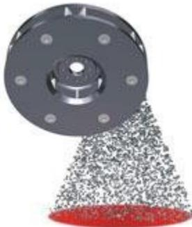
When wear occurs such as the thinning of the blades / vanes or a widening of the aperture in the impellor, the difference in the blast pattern can quickly exceed a change of 20%. This will lead to an increased blast cleaning time, decreased production output and unnecessary wear to the blast chamber. This condition leads to greater abrasive usage caused by the blast stream firing onto the chamber wear plates causing unnecessary abrasive
